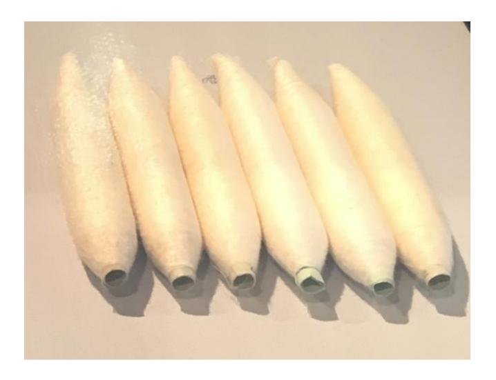
The spinning mule twisted cotton into yarn, then wound it into cones called cops.
