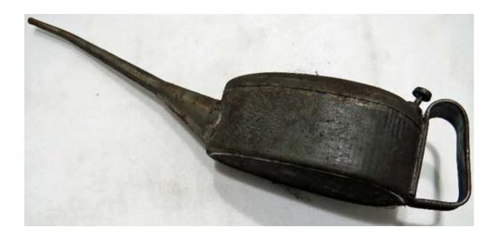
Workers used oil cans to keep the mill machines' moving parts running smoothly.
